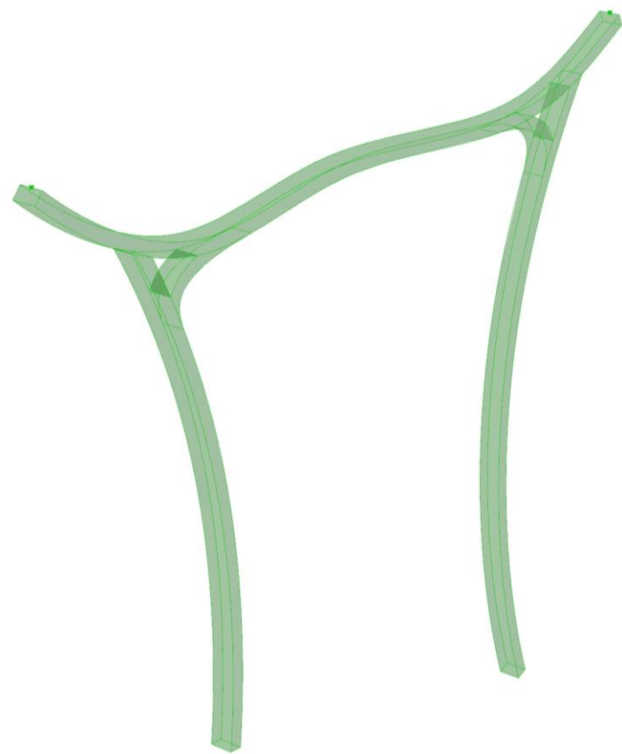
STEP 3 THE LINES GET EXTRUDED A VARIABLE AMOUNT AND OVERHANGS GET TRIMMED AWAY
